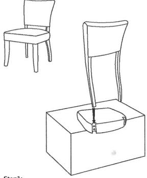
Put the seat pad on the table(height > 50cm), insert the rear legs to the seat gap and move down till hole to hole, Screw the bolts.
